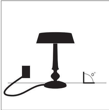
The lamp base should be mounted horizontally on a flat and sturdy surface, preferred accuracy better than 1°. Plug in the power supply.
