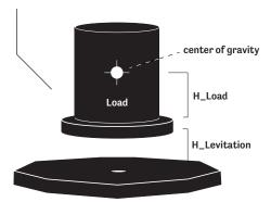
Maximum load location on top of carrier ring:
