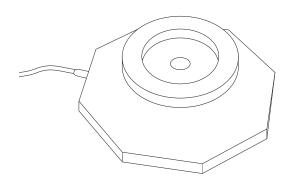
**45** <sup>mm</sup> floating height (max) middle weight **■** (max 1 kg)
